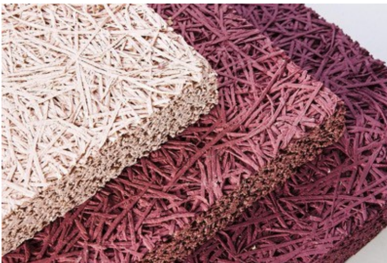
Figure 4-11. Wood Wool Cement Board Product
